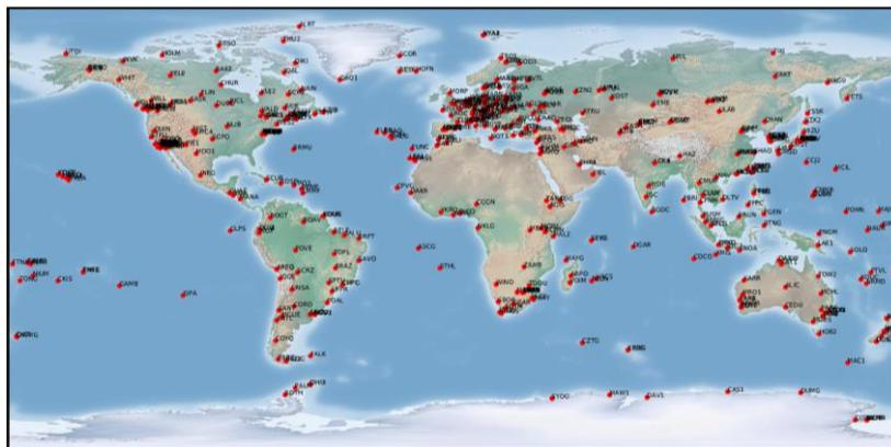
**Figure 1.** Distribution of IGS stations based on GPS Constellation, which has the ITRF2014 coordinates (IGS, 2020)
