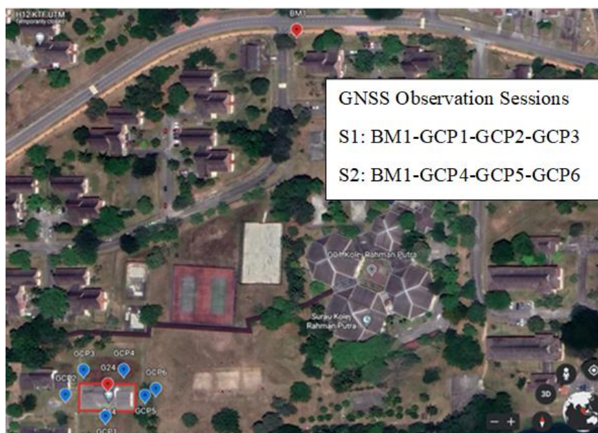
Figure 8. GNSS observation session for GCPs establishment
