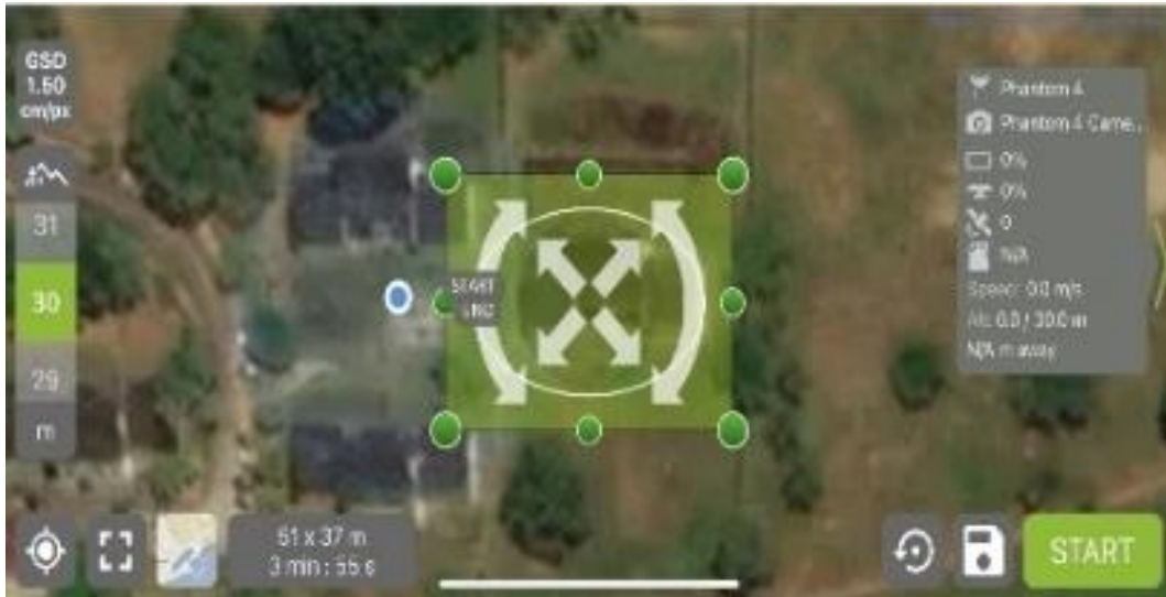
Figure 7. Oblique flight planning using Pix4Dcapture software
