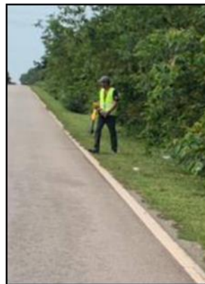
Figure 7. Finding tracing wire by the locator
