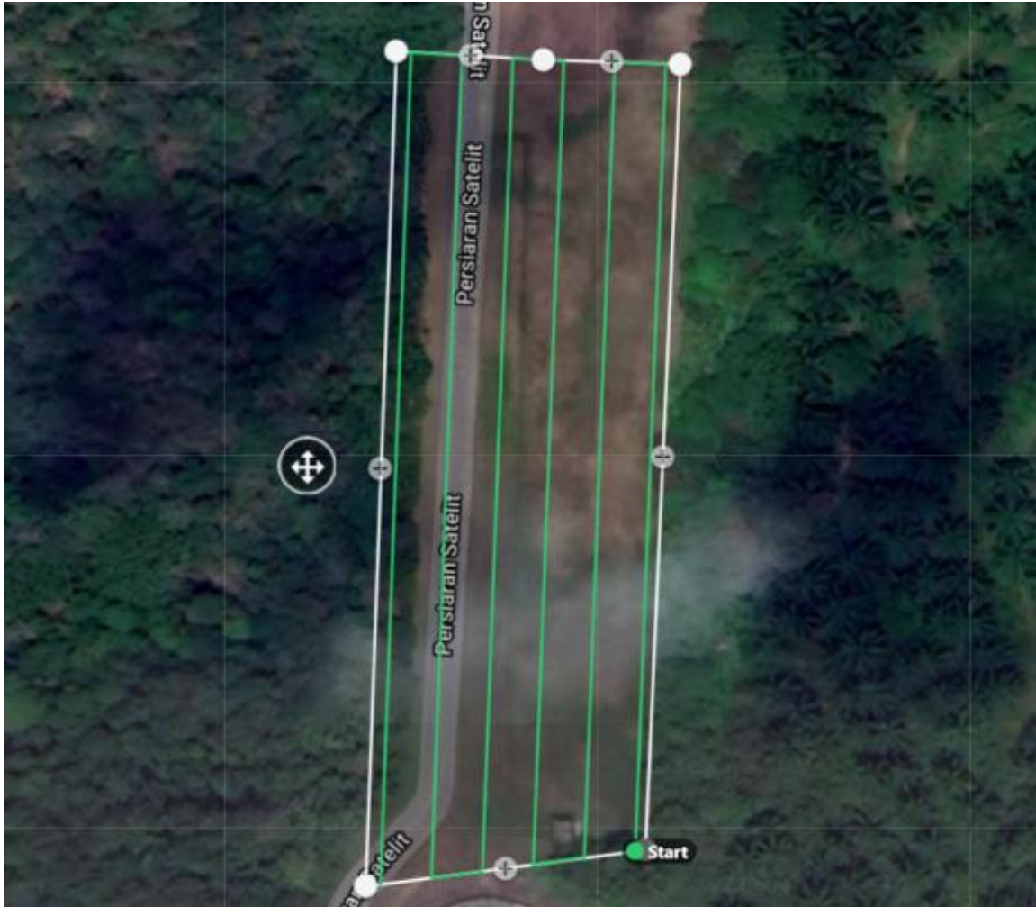
Figure 4. The flight path of UAV in DroneDeploy
