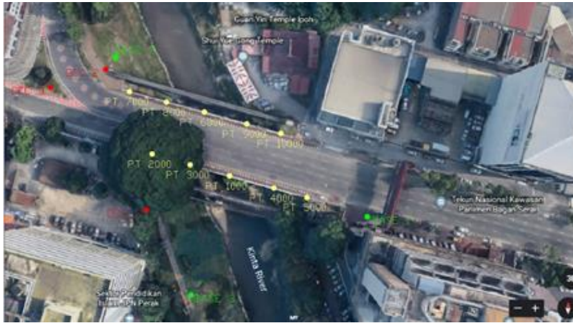
Figure 6. Position of Base Station, Occupy station and Monitoring Points.
